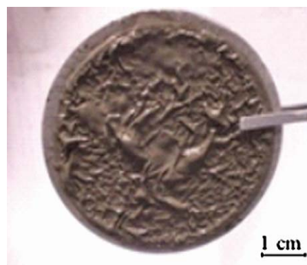
Figure 5 Image of the polymer film observed between the cement filter cake and the sieve after performing the HTHP filtration test using 0.5% bwoc PVA at 27°C. [Color figure can be viewed in the online issue, which is available at www.interscience.wiley.com .]
